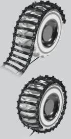
**TRACK TENSION:** The removal of one full track plate may be required to obtain the correct tension. This may be dependent upon whether the track is fitted to new or worn tyre.
