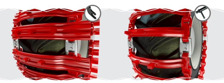
**NOTE:** Fitting these links the wrong way round can result in tyre damage. Tyres MUST be run at correct pressure, check manufactures recommendations.
